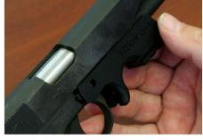
STEP 3 - SLIDE THE TICK DOWN THE FRAME AND OVER THE ELONGATED SSP. THE SSP MUST PROTRUDE THROUGH THE HOLE IN THE ARM OF THE TICK (TO ENSURE A SNUG FIT, RESS DOWN ON THE ARM OF THE TICK)
